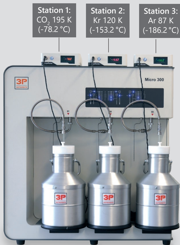
Figure 6 Three different gases on three different ports: the cryoTunes 195, 120 and 87 on a 3P micro 300 micropore analyzer
